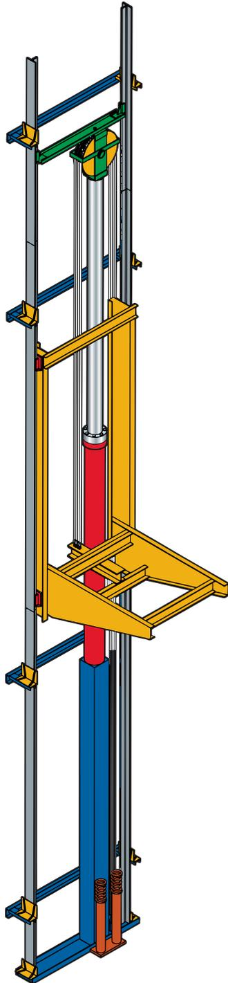
The Cantilever Roped Hydraulic is a holeless elevator that will serve between 25'-0" and 80'-0" of travel (or more under special conditions). They are manufactured in both 2000-lb. and 2500-lb. capacities.
